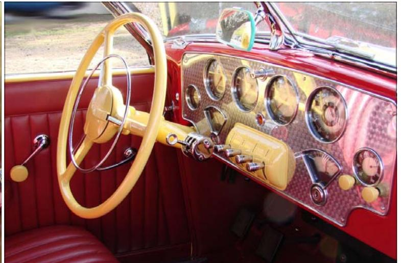
Clockwise from top: The Cord with its “eyes” (headlights) open; the stone shield on the rear bumper; the dash showing the speedometer, odometer, trip odometer, ammeter, temperature gauge, oil pressure gauge, combination fuel and oil level gauge, electric clock and radio; awards won by Ed’s Cord; the open door shows leather upholstery; the touch gearshift—move the knob to the desired gear, depress the clutch and it shifts (behind is the fuel/oil gauge).
