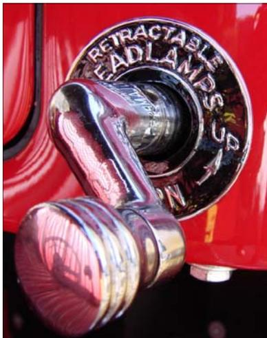
The passenger side hand crank on the dash for the Cord headlights.
