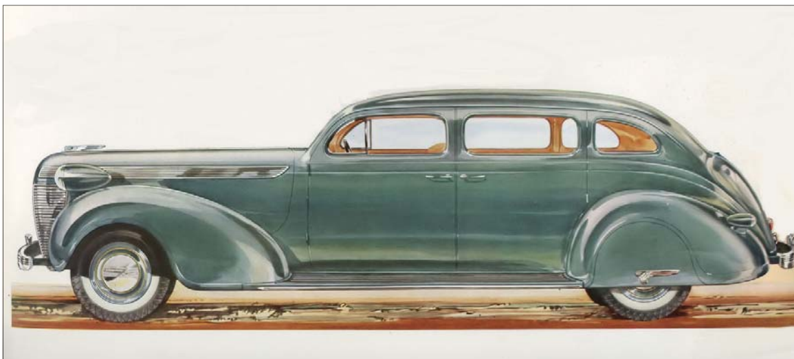
The 1937 Chrysler Custom Imperial 7 passenger sedan and sedan limousine (with the optional divider window.) Prices were $2,060 and $2,160 respectively. The wheelbase was 140 inches. Horsepower was 130 standard or 138 optional at 3400 rpm. Displacement of the engine was 323.5 inches with 6.2:1 or optional 6.5:1 compression ratio. These were all considered factory semi-custom. Also available on special order were custom cars by LeBaron or Derham.
