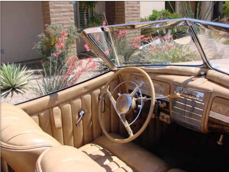
Note the padded dash top area on the 1941 Darrin Convertible Victoria. This car has both Aero-drive and the Electro-mechanical clutch accessories.
