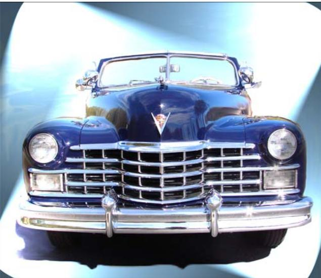
In 1947 the standard turn/parking lamps were small and round. This car has the optional lamps with 3 filaments including the fog lamps.
