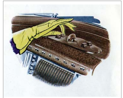
The 1941 Chrysler Crown Imperial sales catalog shows a woman's gloved hand adjusting the front electric windows with a switch on the dash.
