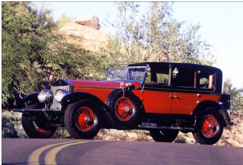
The Roamer 4 passenger Special Sport Series 8-88 for 1929. Note the dual windshield with side sections, and the flaps at the rear of the front fenders. This Roamer did not have running boards, but did have step plates. Tires were 6.50 x 20 and wheels were spoke, wood or disc.
