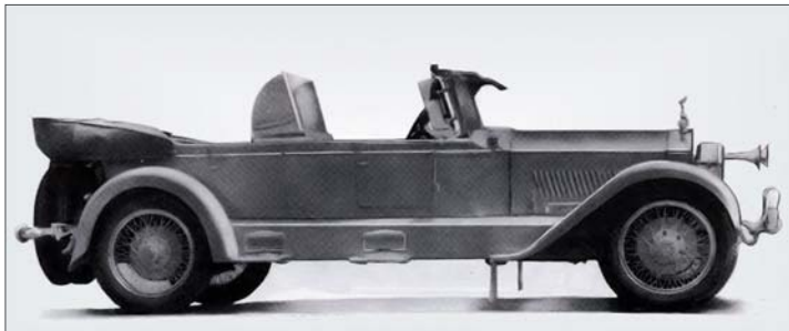
The Roamer 4 passenger Special Sport Series 8-88 for 1929. Note the dual windshield with side sections, and the flaps at the rear of the front fenders. This Roamer did not have running boards, but did have step plates. Tires were 6.50 x 20 and wheels were spoke, wood or disc.
