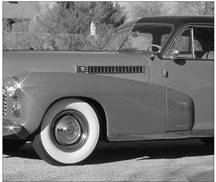
The front fenders of the 1941 Cadillac 60 special extended into the front doors. This is believed to be the first time this design was used on an American built car.
